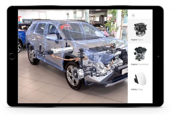
If the tracking is successful, the 3D model snaps to the car and the UI menu will be visible
